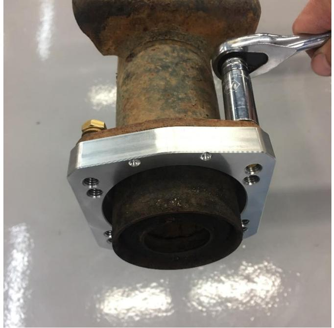
Make sure the surface of the axle flange is clean and deburred before installing the spacer. Install the machined spacer using the hardware provided in the top 2 axle flange holes as shown. The dimples will be mounted **UP** and **OUT** when installed properly. The 10" axle flange adapter is shown in these pics. **If you have the 11" axle flange adapter**, all 4 mounting bolts will start from the outside and go into your axle flange.
