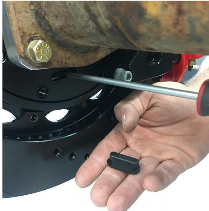
Adjust the parking brake shoes outward using a drum shoe adjustment tool (available at your local parts store) or a flat head screwdriver. You'll do this by spinning the rotor slowly until a slight drag is felt against the hat/drum. The rotor will need lug nuts installed while doing this so that it remains fully seated against the axle shaft.
