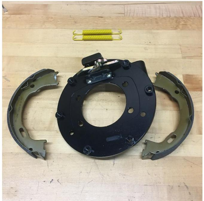
Remove the tensioner and the remaining springs from the assembly so that you have access to the backing plate.
