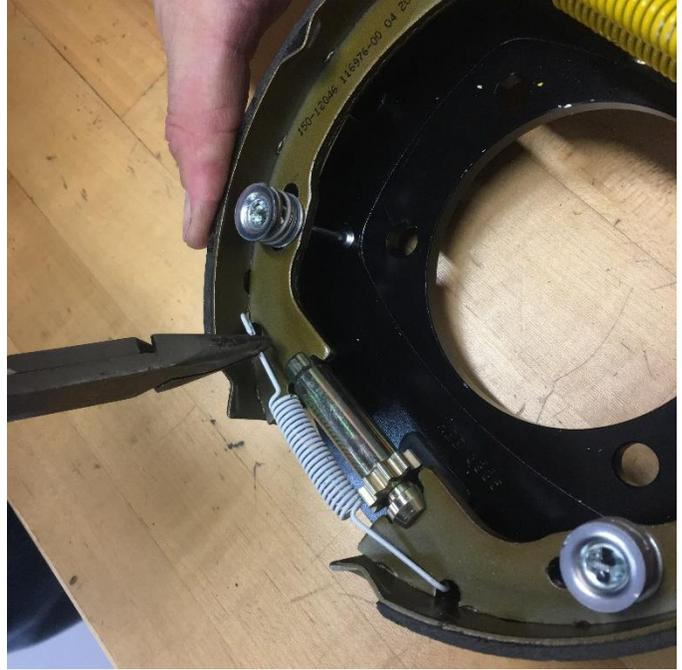
Reinstall the shoe retaining springs as shown, and then finish by reinstalling the bottom spring over the adjuster. At this time, the adjuster should be in the innermost position but not be bottomed out and difficult to adjust through the slotted window after assembly.
