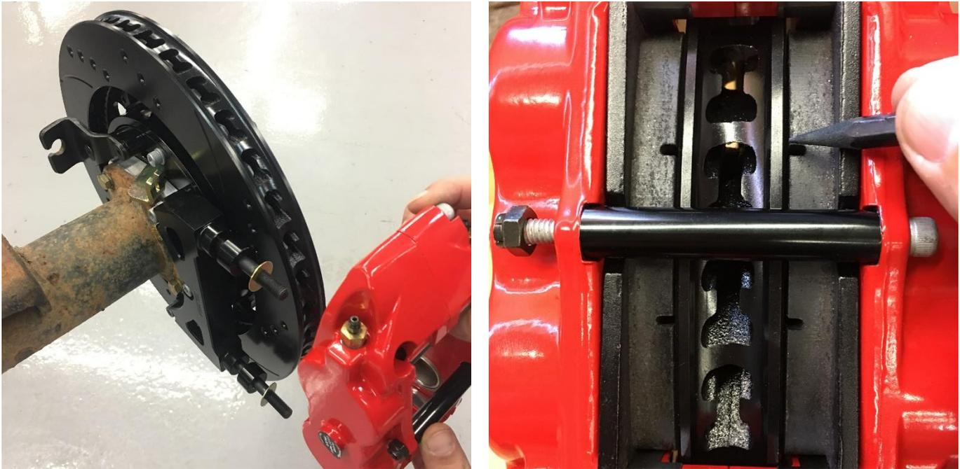
Lubricate the caliper mounting studs with lightweight oil. Initially place one .875x.375x.035 shim on each stud of the bracket. Mount the caliper using lock nuts and washers and ensure that it fully seats on the bracket and does not contact the rotor.
