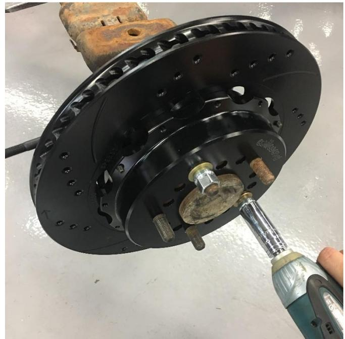
Arrange the rotor and hat in the position shown ensuring the arrow noting rotation direction is correct for its position on the vehicle. Start the first few threads of all 12 of the 1/4-20 x .75 12-point bolts. Using an alternating sequence, apply red Loctite® 271 to the threads, and torque to **155 in-lbs**. The rotor can now be installed using 2 lug nuts to temporarily secure it. Make sure that there is no drag from the parking brake shoes on the rotor at this time.
