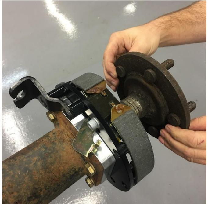
The parking brake assembly can now be installed onto the axle with the supplied hardware. The axle shaft can now be reinstalled per OEM recommendations.
