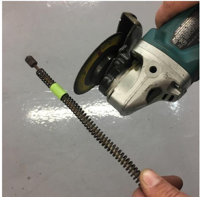
Install the stock parking brake cable into the bracket to hold cable in place. Mark the cable and spring to be cut beyond the cable stop by 1". Use a cut off wheel or cable cutters to cut the cable to the desired length.
