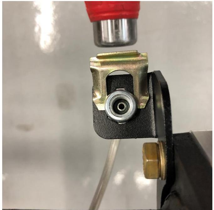
Install the stainless hose onto the caliper fitting. The hose will be routed under the axle and through the hose bracket. Install the retaining clip as shown, being careful not to bend the hose bracket. The factory brake hardline can then be rerouted into the top side of your brake line bracket and tightened into the braided hose.
