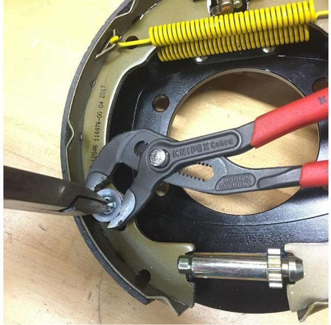
When using the stock parking brake cables, you will need to disassemble the parking brake assembly to install a new cable bracket. Your new levers are included separately. If you purchased our [Parking Brake Cable Kit](#), steps 12-20 are **NOT** required. To swap them out, start by removing the retention springs as shown.
