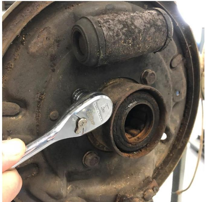
The axles will need to be removed from the housing by draining the fluid, then removing the differential cover, cross pin, and C-clip retainers. The 4 bolts retaining the drum backing plate to the axle can now be removed and discarded.
